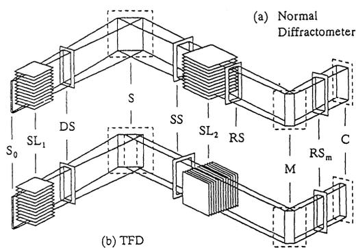
Fig.1 Optical arrangement of normal diffractometer(a) and TFD(b).
